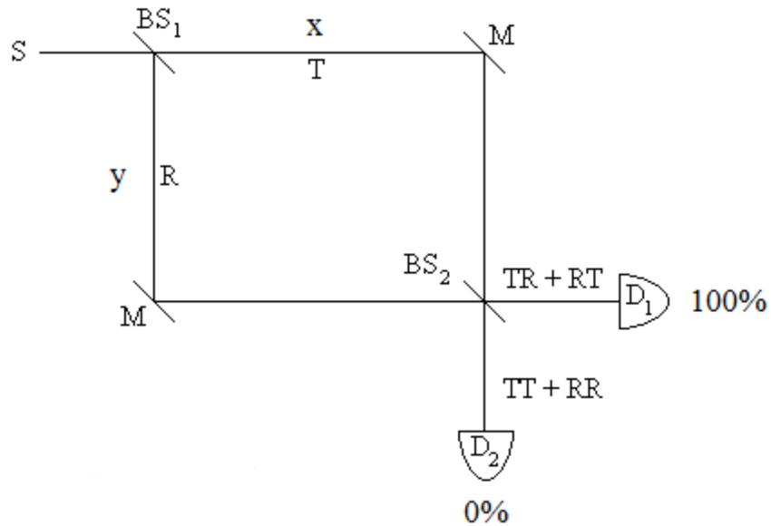
The mathematics of this approach is described below. After the first beam splitter the photon is in superposition of being transmitted and reflected.
