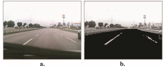
Figure 9. Area detection: (a) Original image; (b) area detected image (pure black fields) (from Yenikaya [13]).
