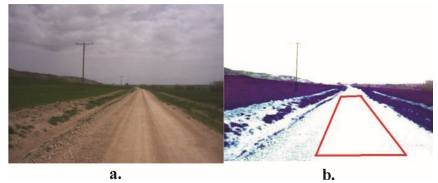
Figure 8. Texture analysis: (a) Original image; (b) refined image (white fields point to the road, blue fields point outside) (from Yenikaya [13]).
