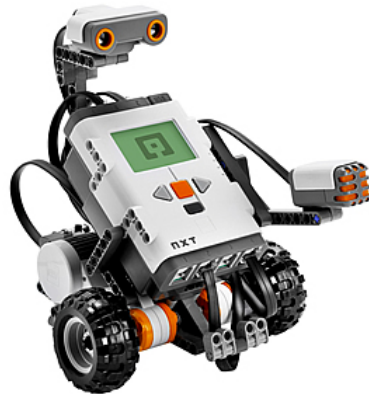
Figure 11. A LEGO Mindstorms NXT robot
